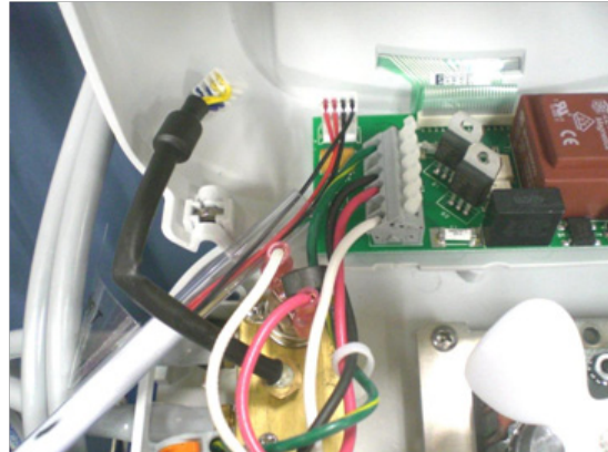
Figure 10: Connection of Test Temperature Sensor
